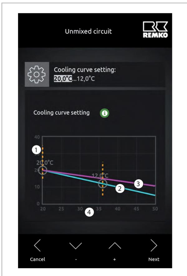
Fig. 7: Cooling curve adjustment
