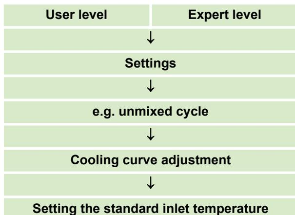
**A cooling function via the cooling curve setting is only enabled by REMKO if the corresponding humidity probe is installed!**
