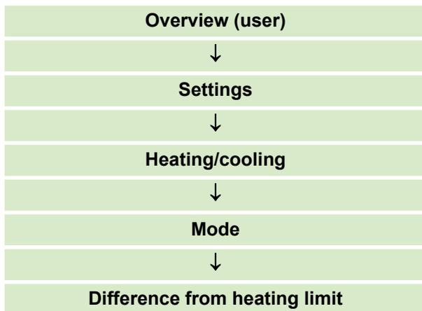
The value 0.0 K means that the heat pump only switches to summer mode if the room set temperature, e.g. 20 °C, is reached at the external probe. Please note the diagram in Fig. 9 for information on which value should be set here.
