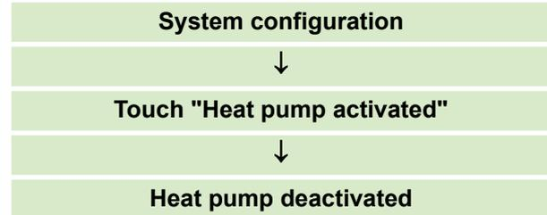
With the deactivation of the heat pump, the Emergency-heat operation via the auxiliary heating is active.
