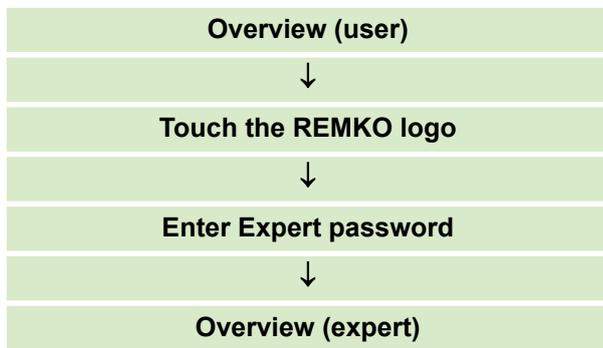
In the expert level, the parameter "Heat pump" can be accessed as follows:
