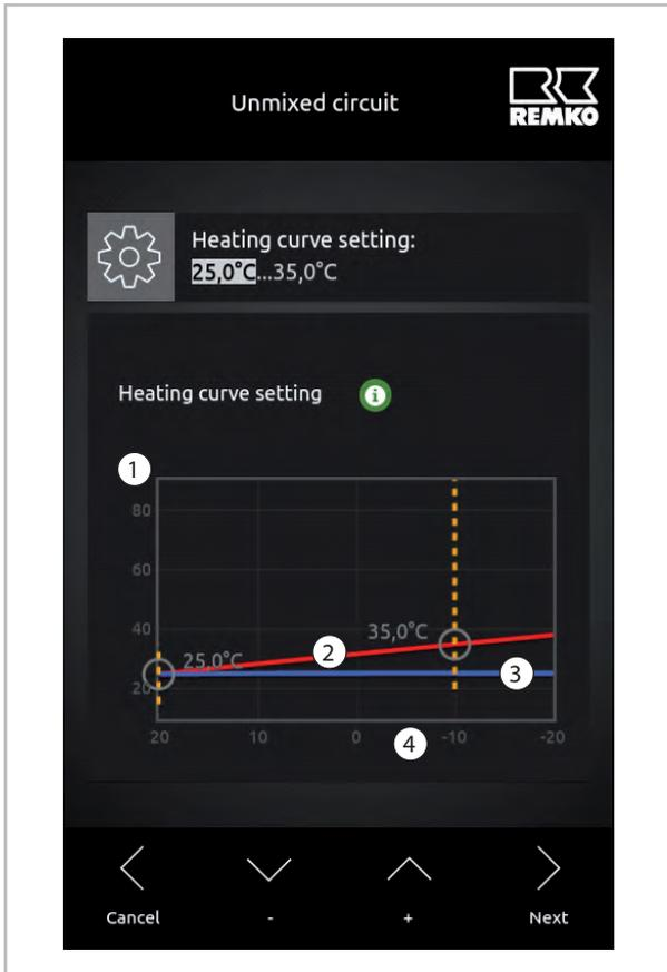
Fig. 6: Heating curve adjustment
