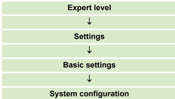
In the "System configuration" level, set the required heating circuit from "deactivated" to "activated". After activation, the circuit is now enabled and can be set in the "User" level and in the "Expert" level of the connected heating circuit configuration. For this purpose, implement the changes as described in the chapter "Setting the heating/cooling operating mode".
