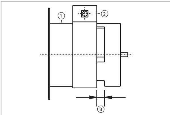
Fig. 3: Setting the air slide
