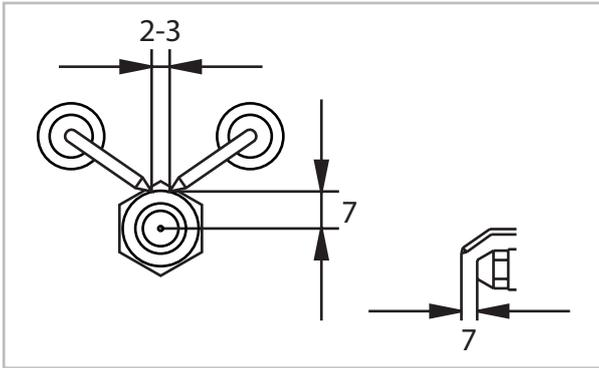
Fig. 2: Setting the ignition electrodes (information approx. values in mm)
