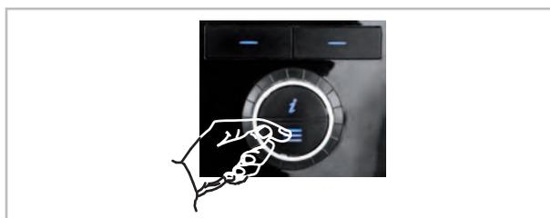
3. ➤ Enter the password "0 3 2 1" by turning the rotary knob and by pressing of the "Next" key.
