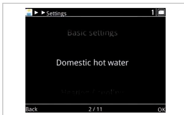
5. ▶ Turn the rotary knob until the parameter "Hygiene function" appears. Press the "OK" key to get to this level.
