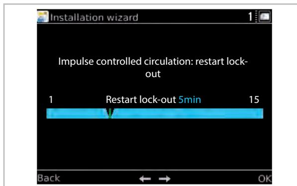
Fig. 46: Impulse-guided circulation - Setting disable switch-on
