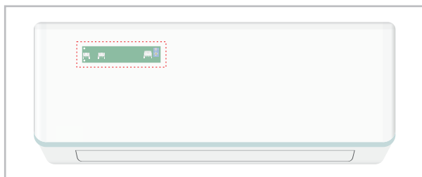
Fig. 45: Installation position of the adapter board
