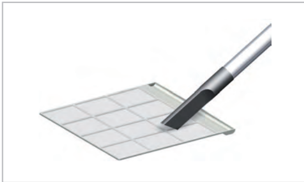
Fig. 22: Cleaning with a vacuum cleaner
