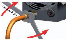
Loosen gas hose: Turn the union nut clockwise
