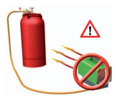
In order to avoid the gas cylinder(s) icing up, it is necessary to configure the gas supply in accordance with the unit connection value, the time in operation and the ambient temperature of the supply tank.
