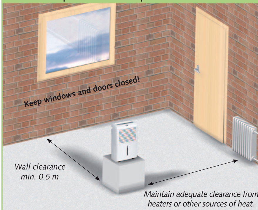
Schematic depiction of how to set up the REMKO air dehumidifier
