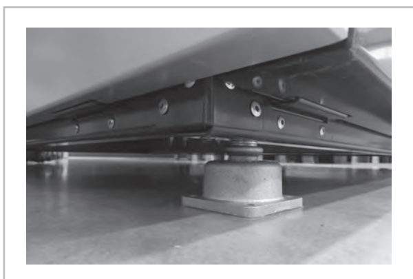
Fig. 20: Vibration dampers mounted
