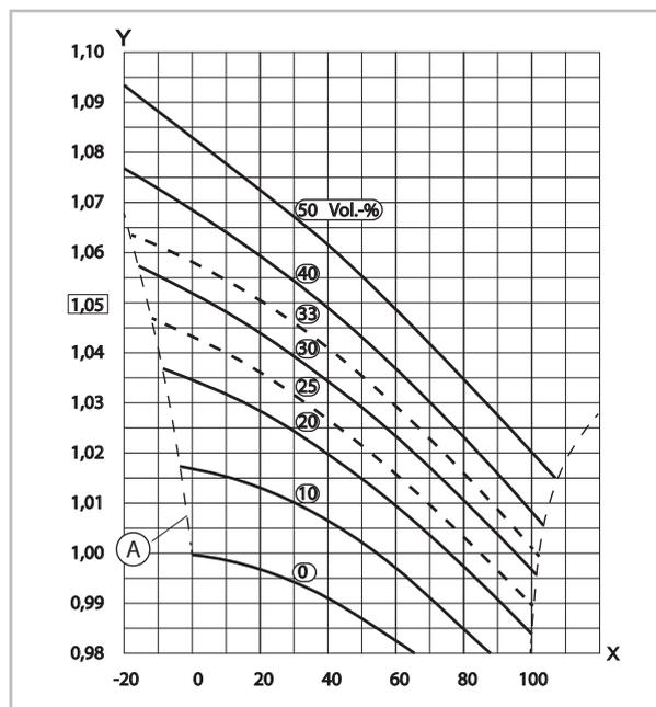
*Fig. 14: Determining brine concentration*
