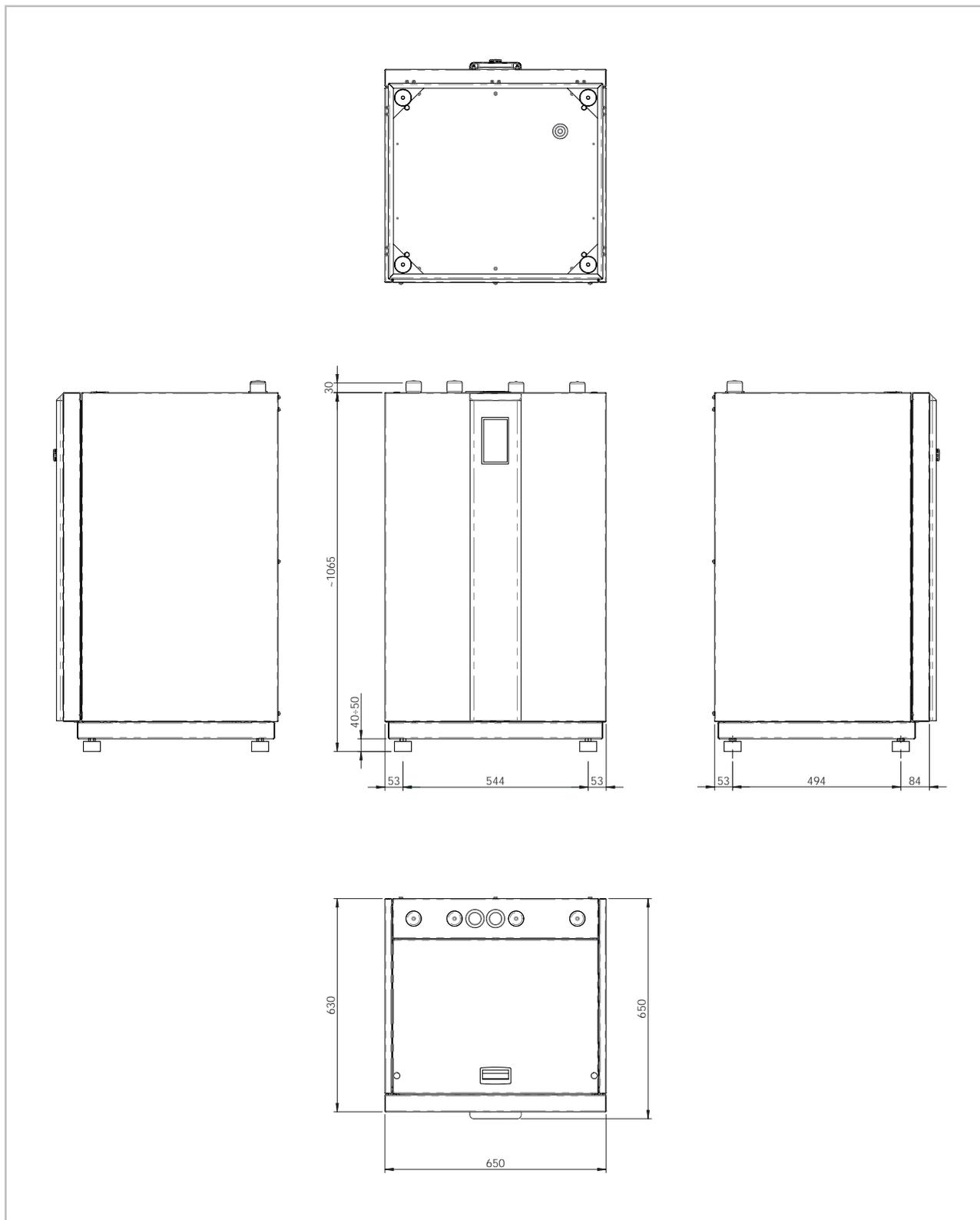
Fig. 1: Heat pump dimensions
