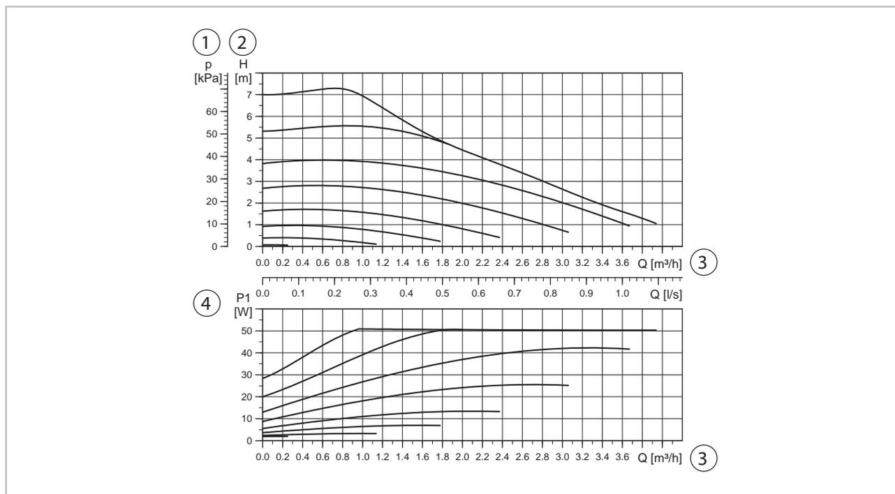
Fig. 5: Circulation pump: Grundfos UPM 3 25-70 130 - capacity range
