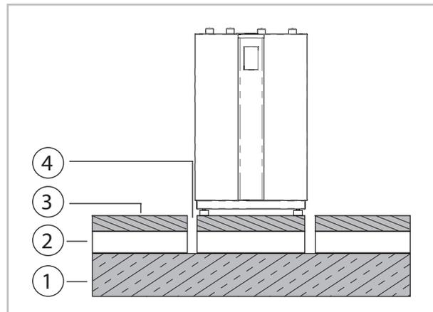
Fig. 13: Decoupling from concrete slab floor
