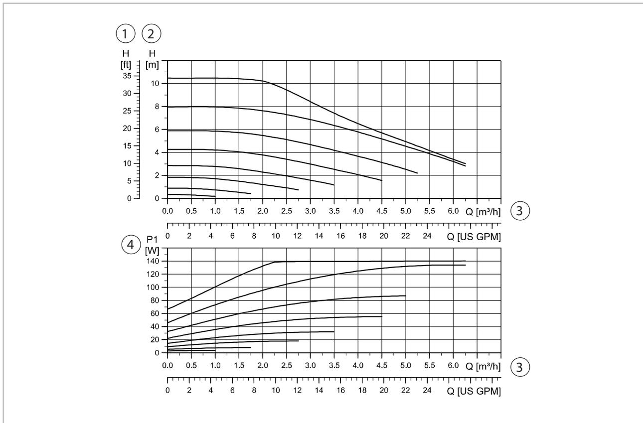
Fig. 6: Circulation pump: Grundfos UPMUPML 15-105 - capacity range
