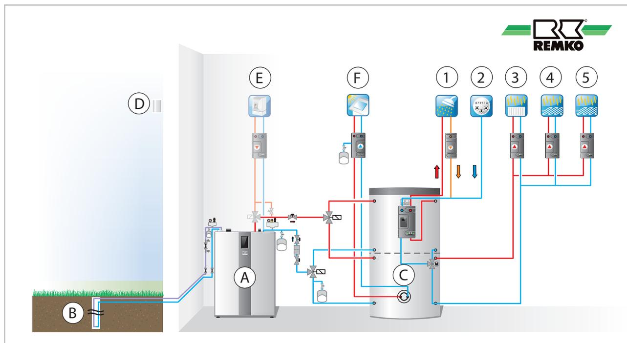
Fig. 18: Example hydraulic cycle diagram WSP\_Solar\_MPS\_011217\_J
