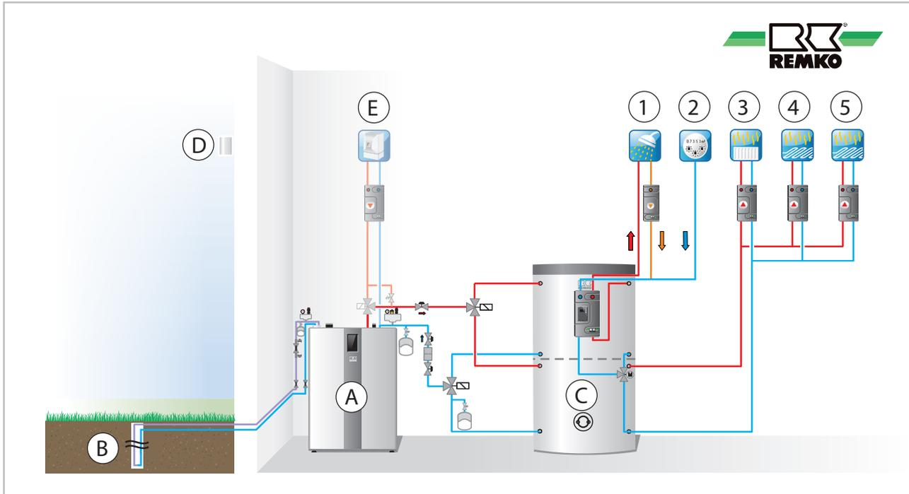
Fig. 17: Example hydraulic cycle diagram WSP\_MPS\_011217\_J
