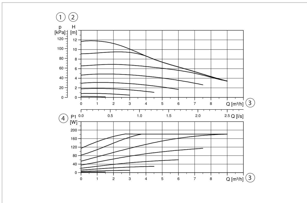
Fig. 7: Circulation pump: Grundfos UPMXXL 25-120 - capacity range
