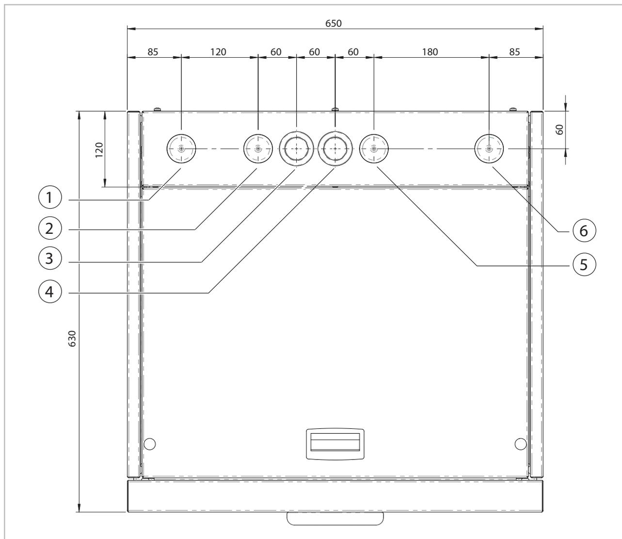
Fig. 2: Designations of pipe connections, plan view
