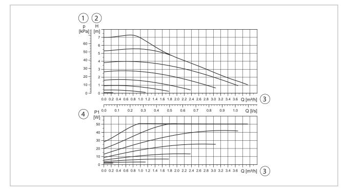
Fig. 5: Circulation pump: Grundfoss UPM 3 25-70 130 - capacity range
