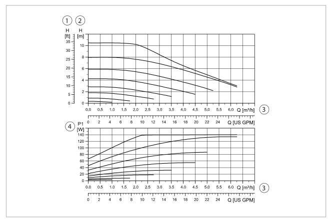
Fig. 6: Circulation pump: Grundfoss UPMUPML 15-105 - capacity range
