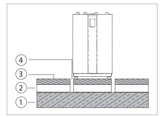
Fig. 13: Decoupling from concrete slab floor
