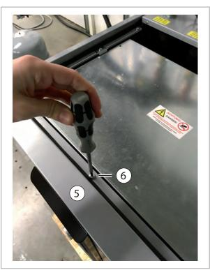
**2.** Then tilt the front door [5] forward and remove it carefully.
