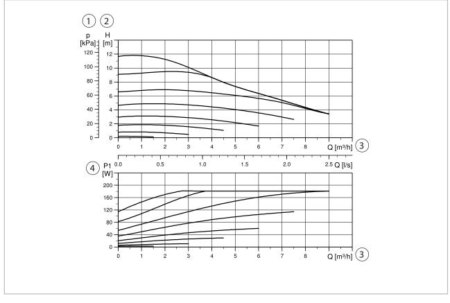
Fig. 7: Circulation pump: Grundfoss UPMXXL 25-120 - capacity range
