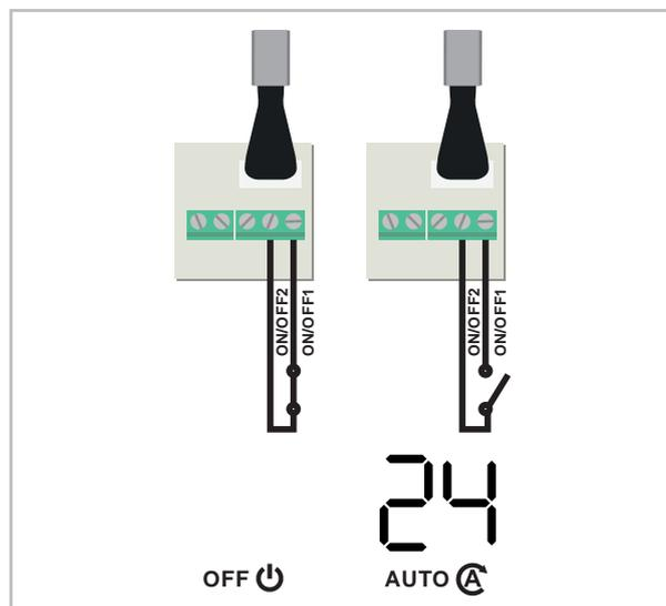
Fig. 52: Borne de raccordement ON/OFF1 & ON/OFF2
