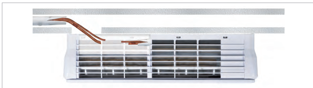
Fig. 31: Under the plaster installation (View from above)
