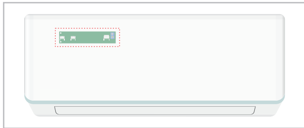
Fig. 48: Installation position of the adapter board
