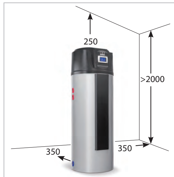
Fig. 8: Minimum distances in mm
